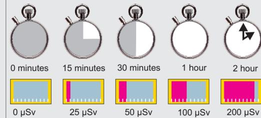
**Distance** If the dose rate at 1 m from a source is 100  $\mu\text{Sv/h}$ , the dose rate at 2 m will be 25  $\mu\text{Sv/h}$ .
