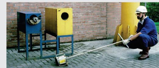
This operator must follow clear procedures for loading a well logging source. The procedures might state that he/she must prevent access to the area while he/she carries out this work, use remote handling tools and complete the task as quickly as possible.
