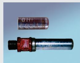
The radioactive material is held within a tough metal casing. The casing prevents the radioactive material from escaping but does not shield the radiation completely.
