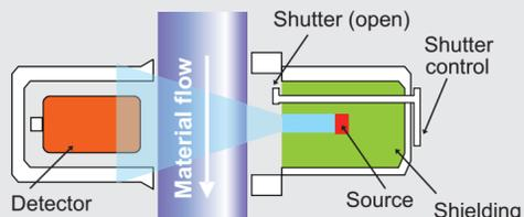
Gamma, beta and neutron radiation sources can all be used in nuclear gauges, depending on the application.
