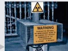
This radioactive source should have been disposed of as radioactive waste. However, it was found in a scrap yard. Appropriate labelling and proper supervision of the source would have prevented this.
