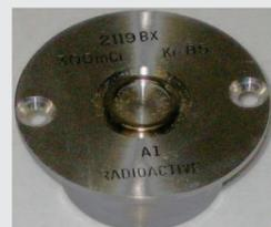
The walls of the capsule are thinner to allow the beta radiation to pass through. Beta sources are usually more fragile than gamma or neutron sources.
