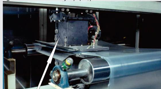
A thickness gauge incorporating a beta source. In the picture above, the source is contained in the housing above the product that is being measured and the detector is on the opposite side.
