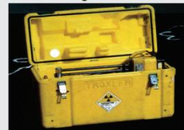
Type A and Type B packages must be labelled to indicate the dose rate on the surface, and at 1 m from the package:
