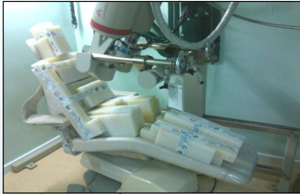
IRSN Brick Phantoms: Female (50 kg), Standard Man (70 kg) and Big Man (90 kg)
