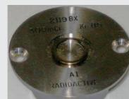
The walls of the capsule are thinner to allow the beta radiation to pass through. Beta sources are usually more fragile than gamma or neutron sources.
