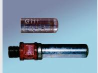
The radioactive material is held within a tough metal casing. The casing prevents the radioactive material from escaping but does not shield the radiation completely.
