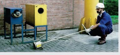
This operator must follow clear procedures for loading a well logging source. The procedures might state that he/she must prevent access to the area while he/she carries out this work, use remote handling tools and complete the task as quickly as possible
