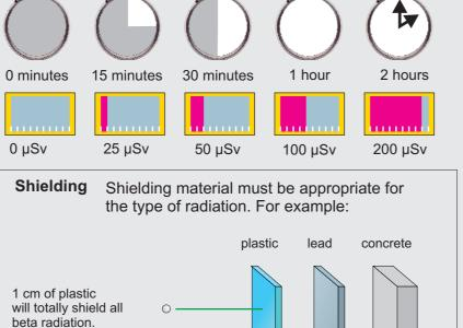
be used to shield against gamma and X radiations. Concrete can also be used to shield against neutron radiation.
