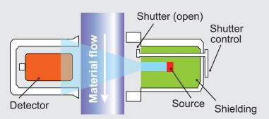
Gamma, beta and neutron radiation sources can all be used in nuclear gauges, depending on the application.
