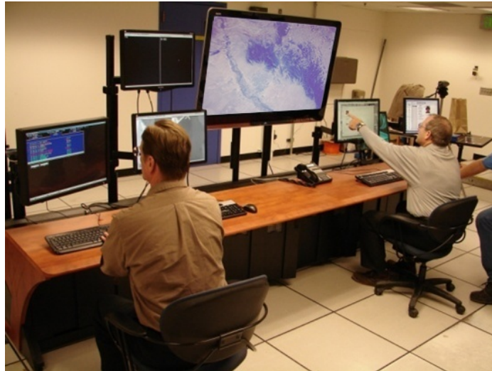
FIG. 16. Example of a layout of a central alarm station workstation.
