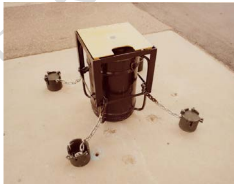
FIG. 48. Additional example of a tie-down device using chains.
