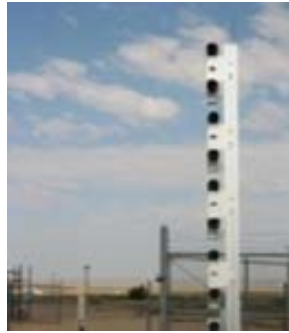
FIG. 6. Active point to point infrared system using multiple beams.
