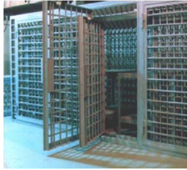
FIG. 46. Example of a double layer steel cage for nuclear material storage.
