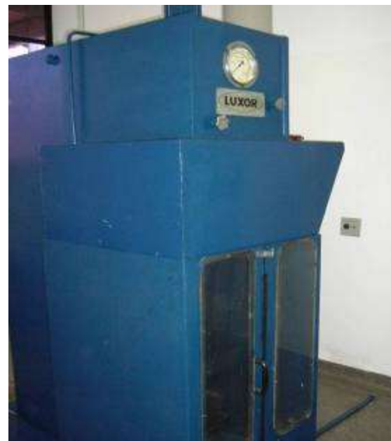
Solid Waste Compaction Equipment - 10.000 kgf, - 5:1
