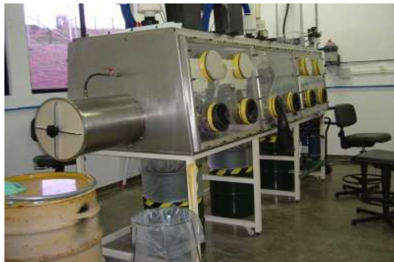
Glove Box for Lightning Rods Dismantling
