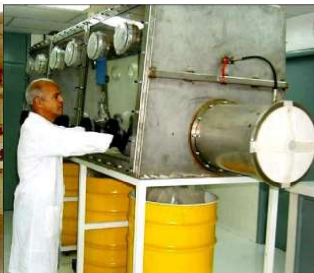
Glove Box for Dismantling of Lightning Rods
