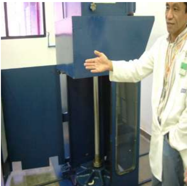
Solid Waste Compaction Equipment - 10.000 kgf, - 5:1
