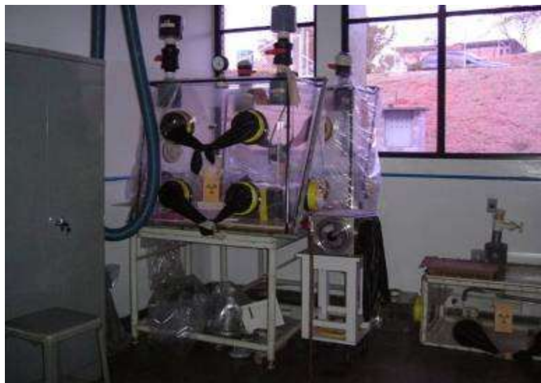
Waste Reception / Segregation Unit
