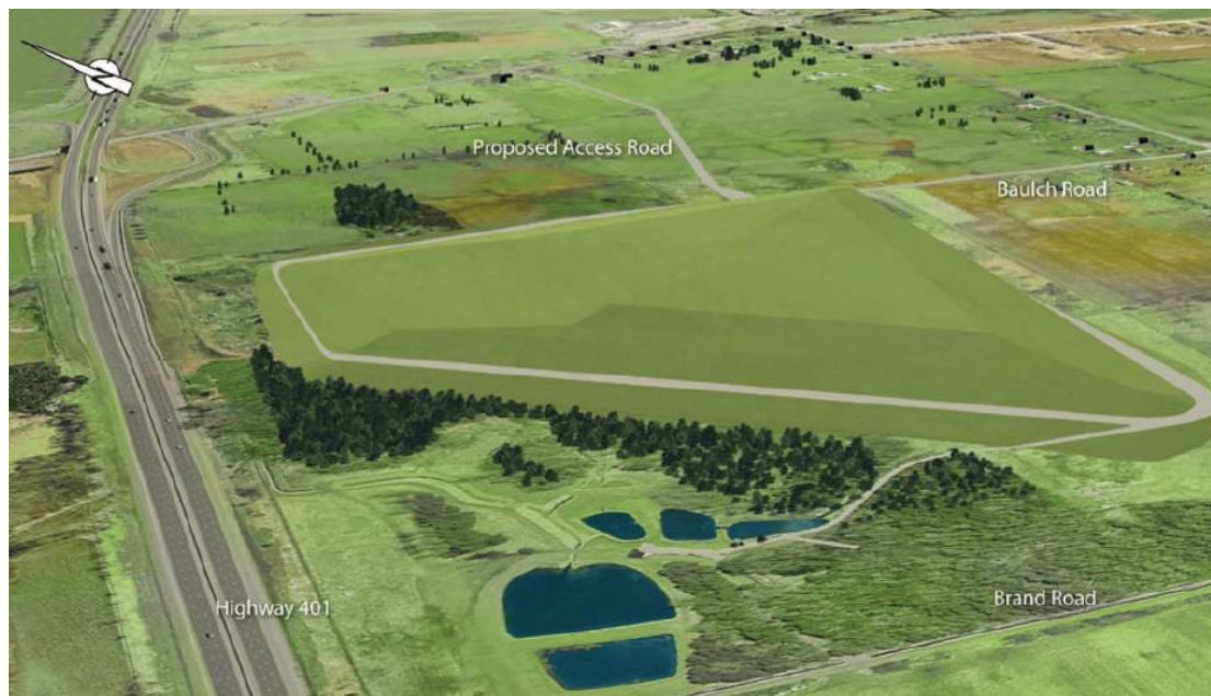
Figure 5.1 Conceptual design for a new above ground, mound type waste management facility for long-lived LLW near Port Hope, Canada.
