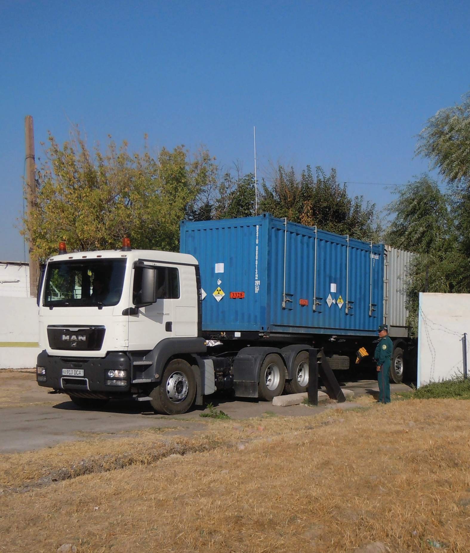
Truck with international standard (ISO) transport container carrying irradiated liquid highly enriched uranium fuel (Uzbekistan).
