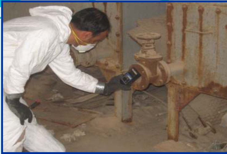
RPC inspector make radiological survey
