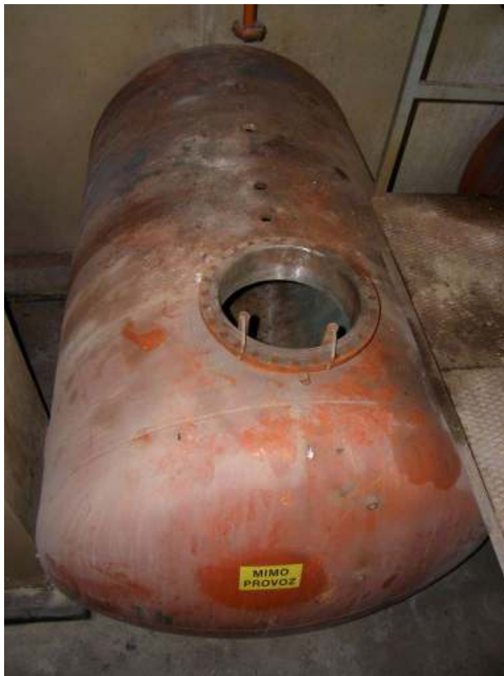
Storage tank before segmentation
