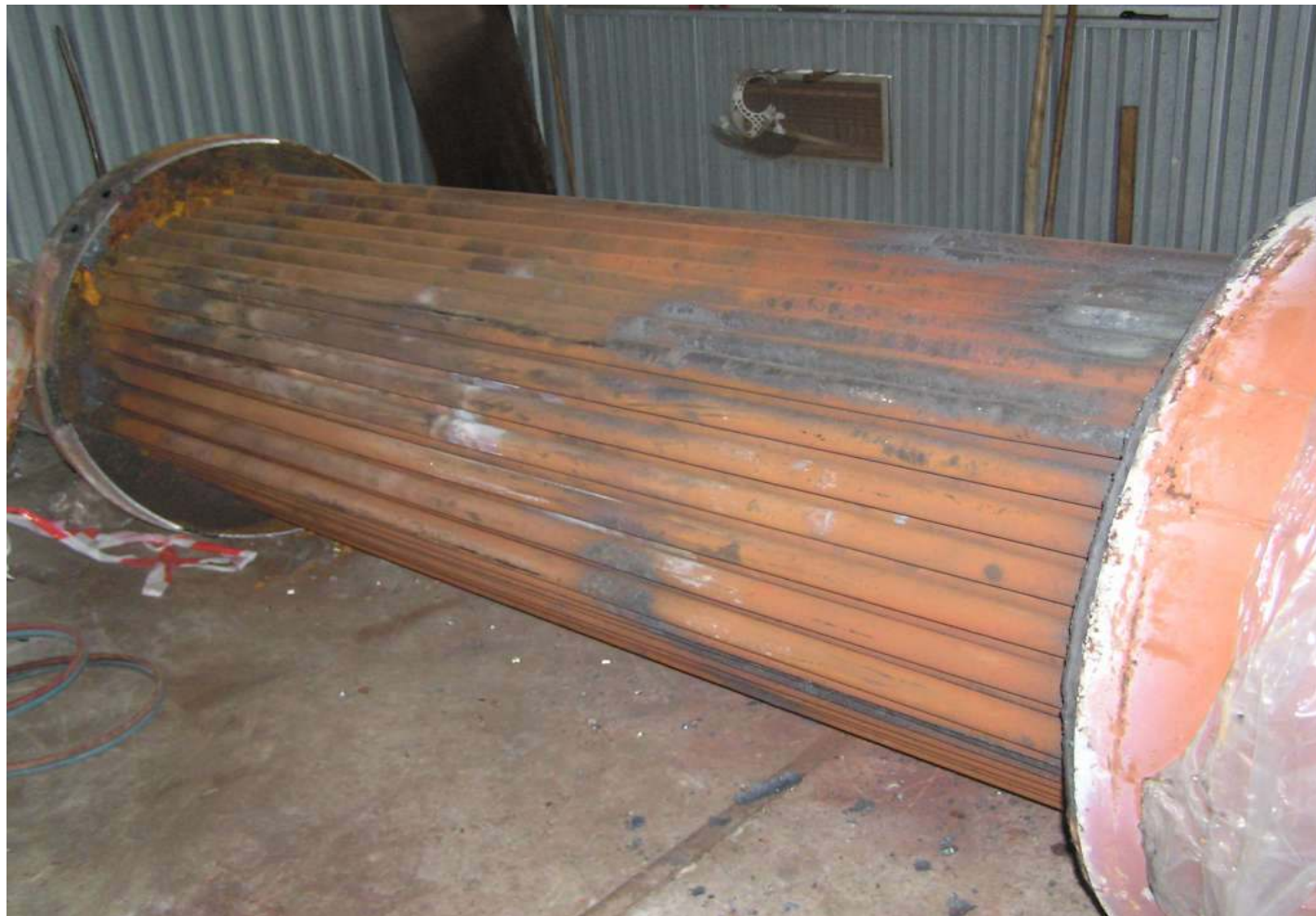
Heat exchanger tubes before segmentation
