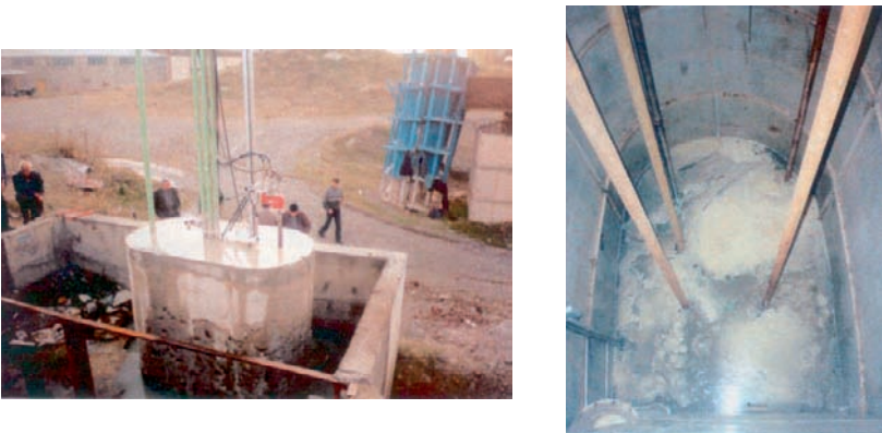
FIG. 9. Mock-up of grouted IRT reactor in Georgia.
