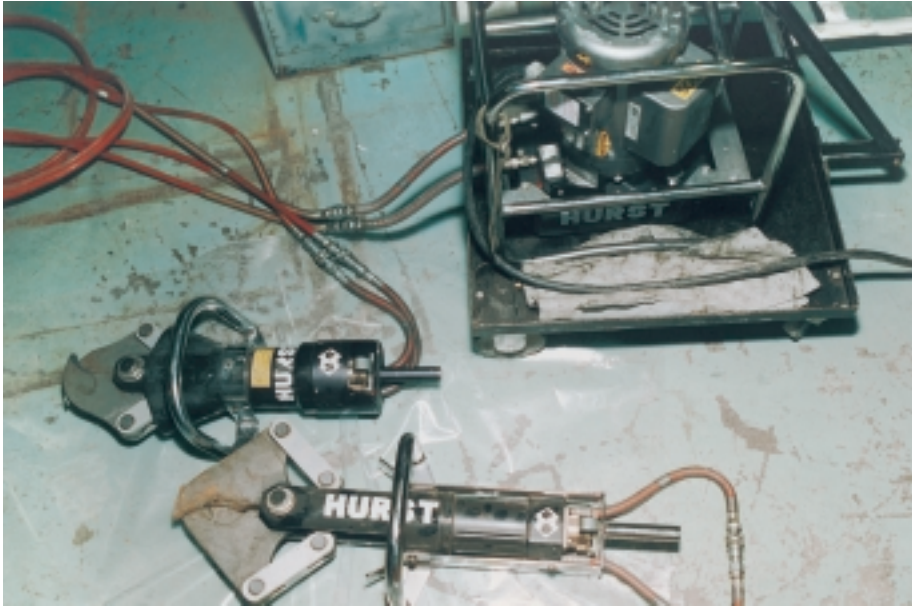
FIG. 15. Pipe cutter used for smaller diameter, tritium contaminated piping. The cutter both cuts and crimps the ends of the pipe. Courtesy Argonne National Laboratory, managed and operated by the University of Chicago for the US Department of Energy under contract No. W-31-109-ENG-38.
