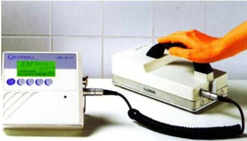
Autonomous recording of the surface contamination through a combined system of the manipulator and a measurement device
