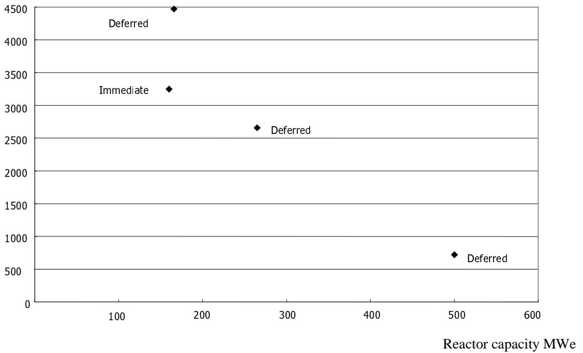
If data sets for all reactor types are considered, specific costs (expressed in USD per kWe) show a slight decreasing trend with increasing capacity. However, this trend is dominated by the high specific costs reported for gas-cooled and small size reactors. If the analysis is limited to water-cooled reactors with capacities higher than 200 MWe, the decreasing trend of specific costs with increase reactor capacity is less significant and the correlation is less robust.
