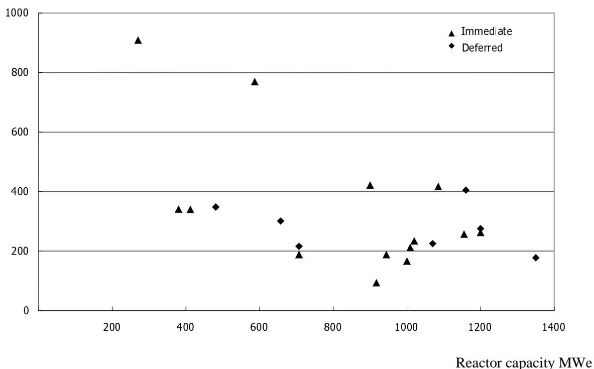
**Figure 4.3. Total Decommissioning Cost (USD 1<sup>st</sup> July 2001/kWe) – VVERs**
