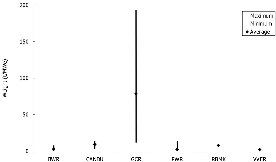
In order to check whether reactor capacity has an effect on waste quantities, the data presented in Figures 2.4 and 2.5 have been normalised, in terms of tonne/MWe, and re-presented in Figures 2.6 and 2.7. These show that reactor capacity is not a determining factor on waste quantities. In addition, it can be seen from Figure 2.6 that the difference between gas-cooled reactors and other reactor types is more marked when considering normalised data.
