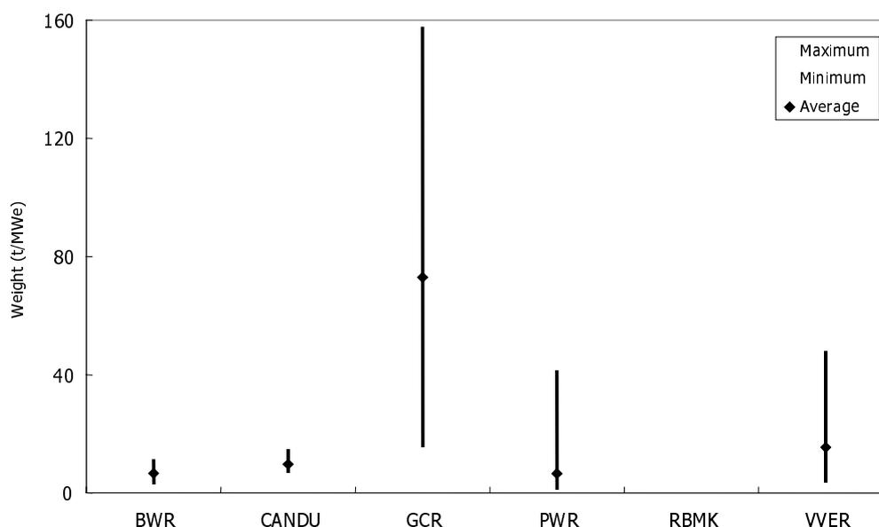
Figure 2.7, which – similarly to Figure 2.5 – presents all radioactive materials shows a greater variability between reactor types, although the gas-cooled reactors are still showing the highest normalised weights. This greater variability between maximum and minimum values probably reflects the differing extent of reactor support facilities and equipment among individual reactors and reactor types.
