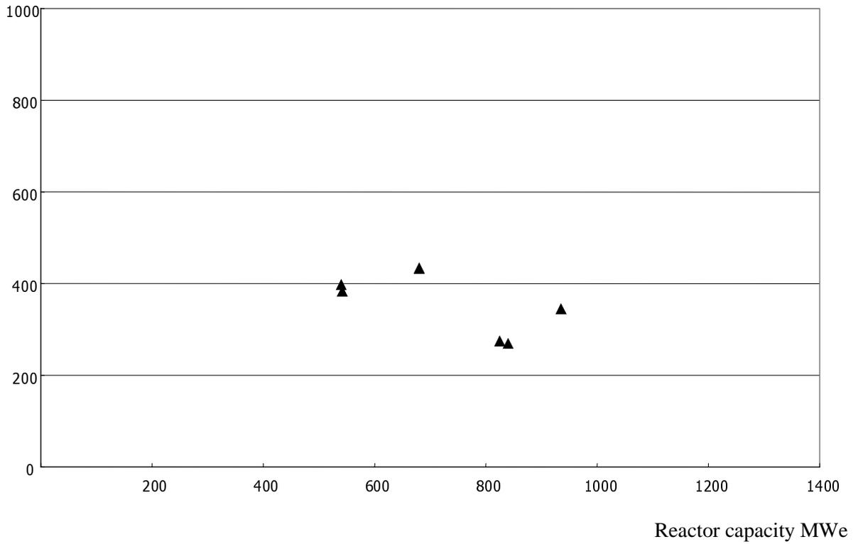
**Figure 4.6. Total Decommissioning Cost (USD 1<sup>st</sup> July 2001/kWe) – GCRs**
