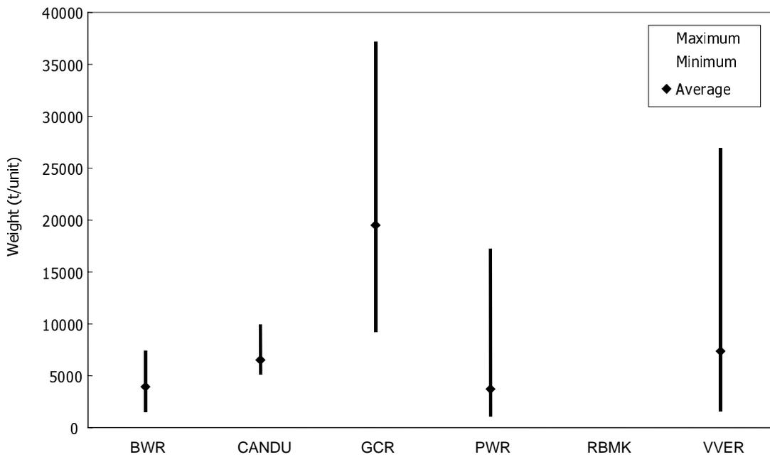
**Figure 2.6. Weight of radioactive reactor materials per MWe**
