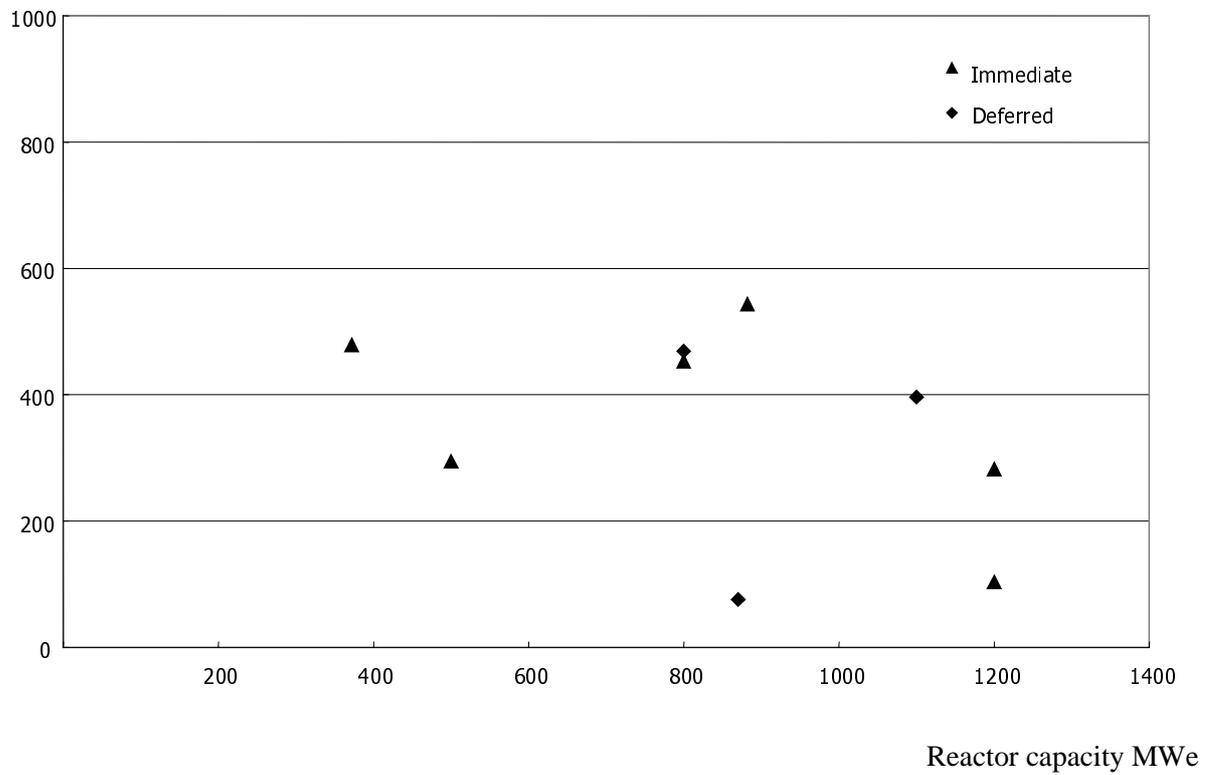
**Figure 4.5. Total Decommissioning Cost (USD 1<sup>st</sup> July 2001/kWe) – PHWRs**
