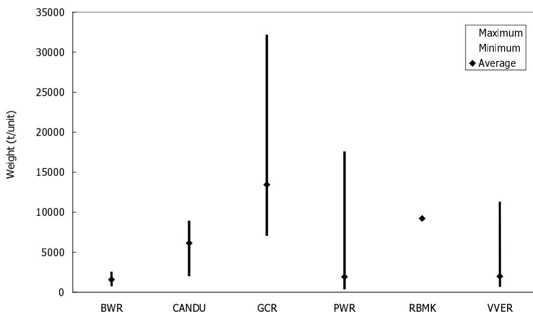
Figure 2.4 relates to the radioactive reactor materials only and shows that gas-cooled reactors (GCRs) produce significantly more radioactive waste than all other reactor types. For all other reactor types, the weight of radioactive reactor materials are generally lower and show less variability within each reactor type.
