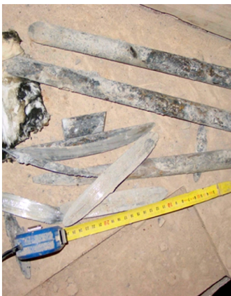
Figure 14. Moon-shaped steel segments cut from reinforcement
