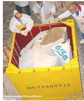
Concrete blocks stored in Konrad Type 2 container
