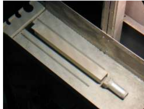
Preparation of a MTR-fuel element for transfer to the Hot Cells
