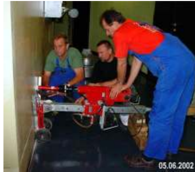
Sampling at the biological shield and the pool liner for „fingerprinting“
