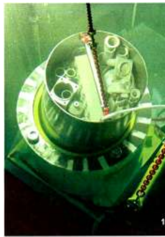
Under water loading of a Mosaik container, activity content 370 GBq Co-60
