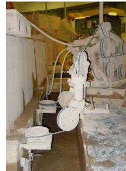
Application of diamond wire cutting saw
