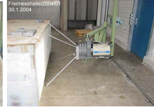
Cleaning the blocks and clearance measurement with a Canberra ISOCS detector
