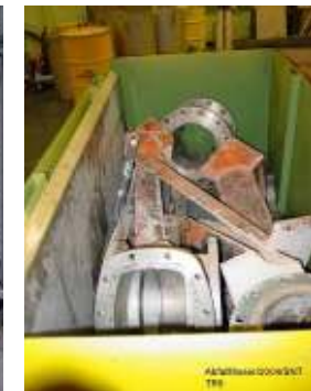
Characterization of metals using ISOCS and collecting metals for further treatment
