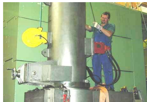
Transfer of a fuel element into the transport flask
