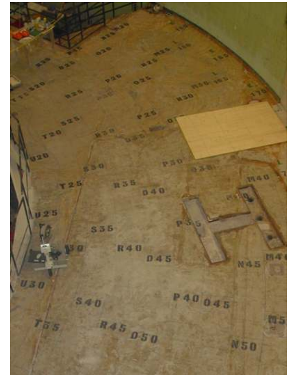
Typical grid pattern at upper floor level to ensure the traceability of measurements
