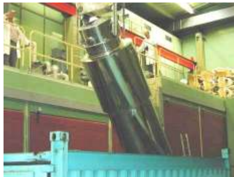
Unloading of a transport flask in the Hot Cell Department
