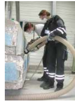
Cleaning the blocks and clearance measurement with a Canberra ISOCS detector
