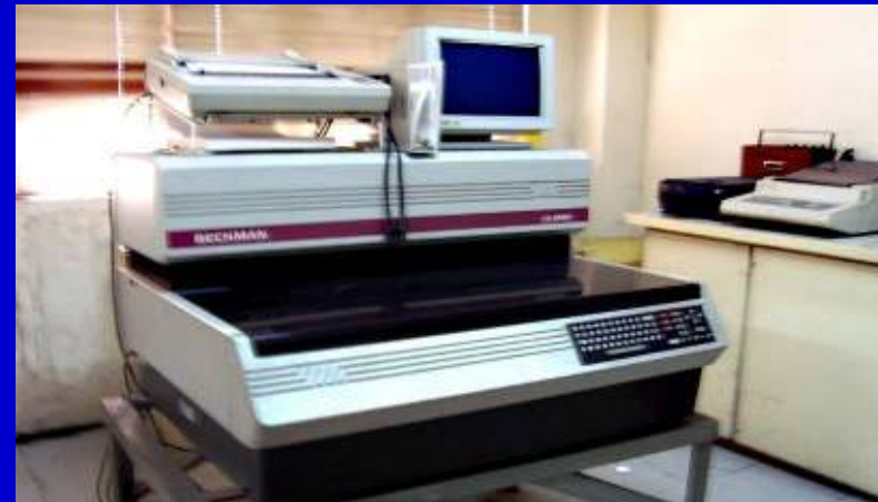
Liquid Scintillation Counter for \beta activity measurement
