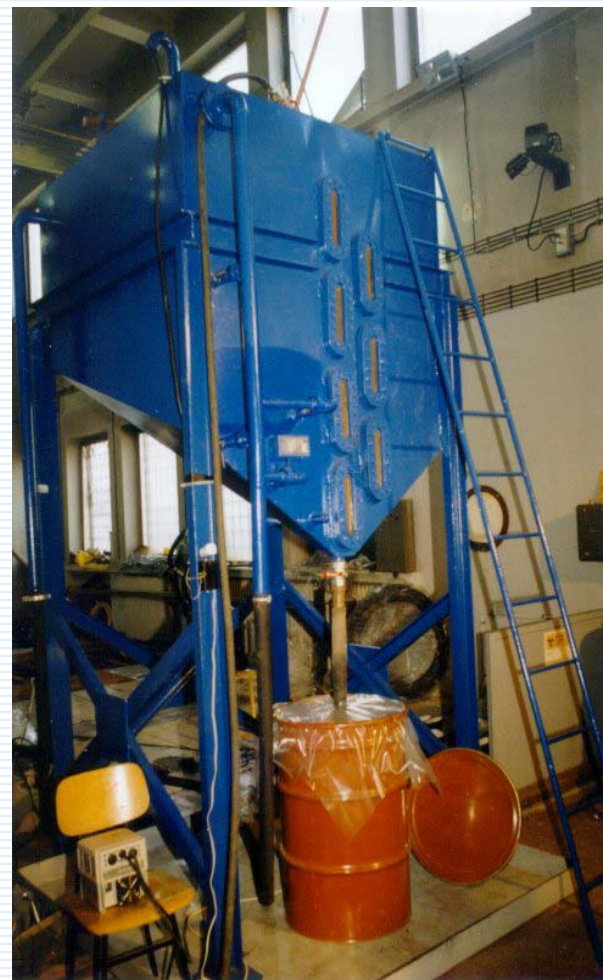
Sedimentation vessel for sludge removal
