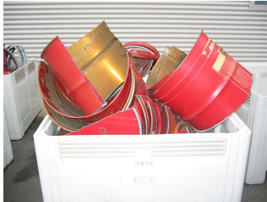
Empty drums cut into section to prevent re-use off site
