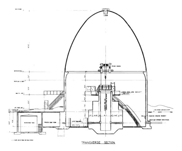
Figure X. Vertical cross section of the reactor building
