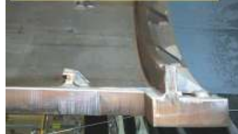
Cutting complex shapes with AWJ
