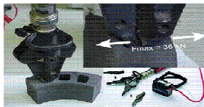
Orbital cutter to dismantle primary piping
