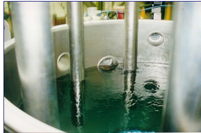
Example of ultrasonic emitters encased in thimble
