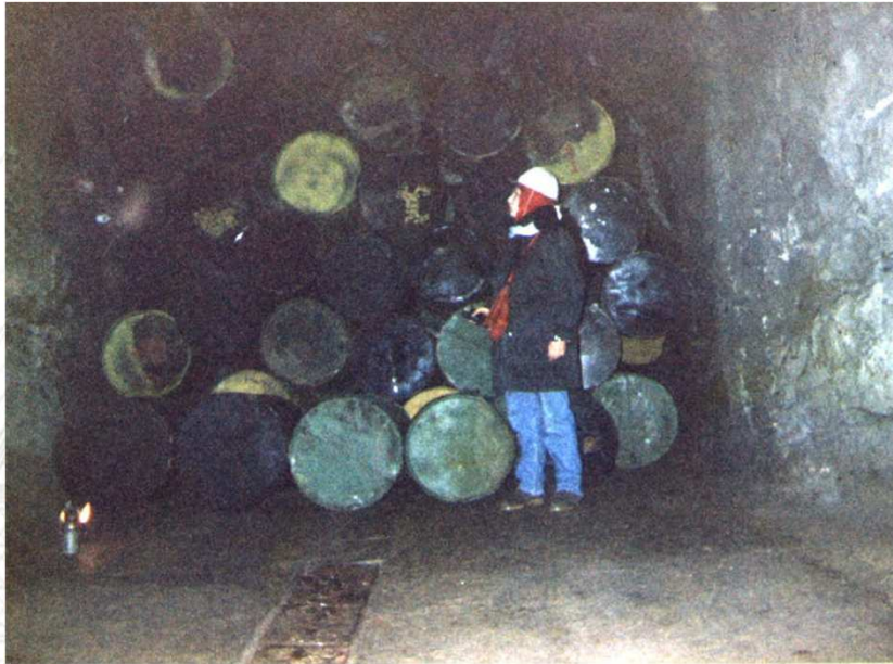
View of Non-backfilled Disposal Gallery showing the Stacking of the Waste Drums
