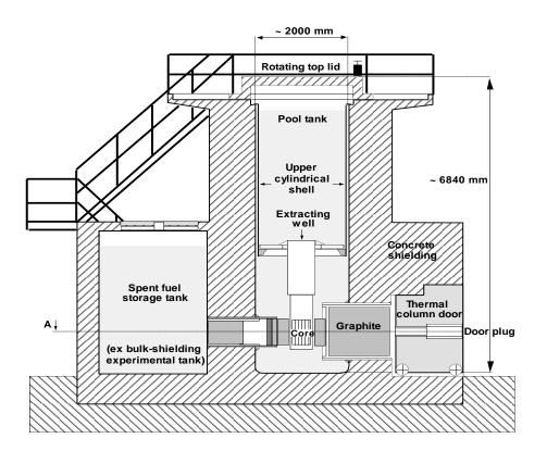
The reactor is installed on the floor at ground elevation in the center of the hall. reactor The reactor tank and major components are surrounded by a thick concrete shielding structure.
