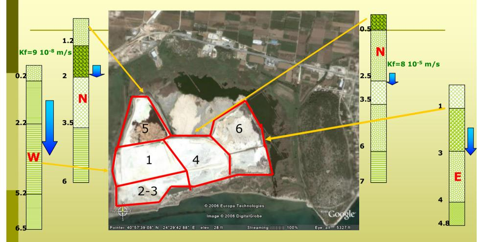
East: clay layer at 4.5m NE, water: 2.1-2.9m, lack of clay layer  $\rightarrow$  underground runoff of the pg drainage to S
