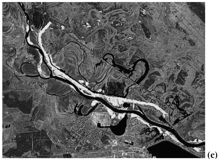
Fig. I.2. Modification of the Pripyat River Floodplain in Chernobyl Exclusion Zone (SPOT Satellite Images). (a) 1986, Original shape; (b) 1994, embankment of the left bank sandy dike; (c) 1999, embankment of the right bank sandy dike.
