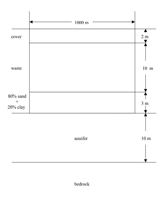
Fig. 1: Vertical scheme of the waste dump
