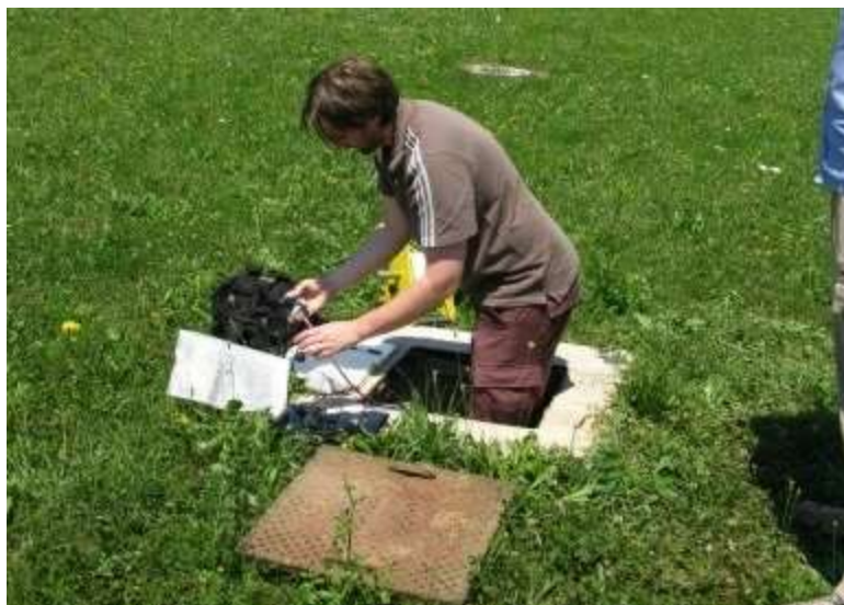
FIG. 22. Borehole system around the CSF is equipped as piezometer.
