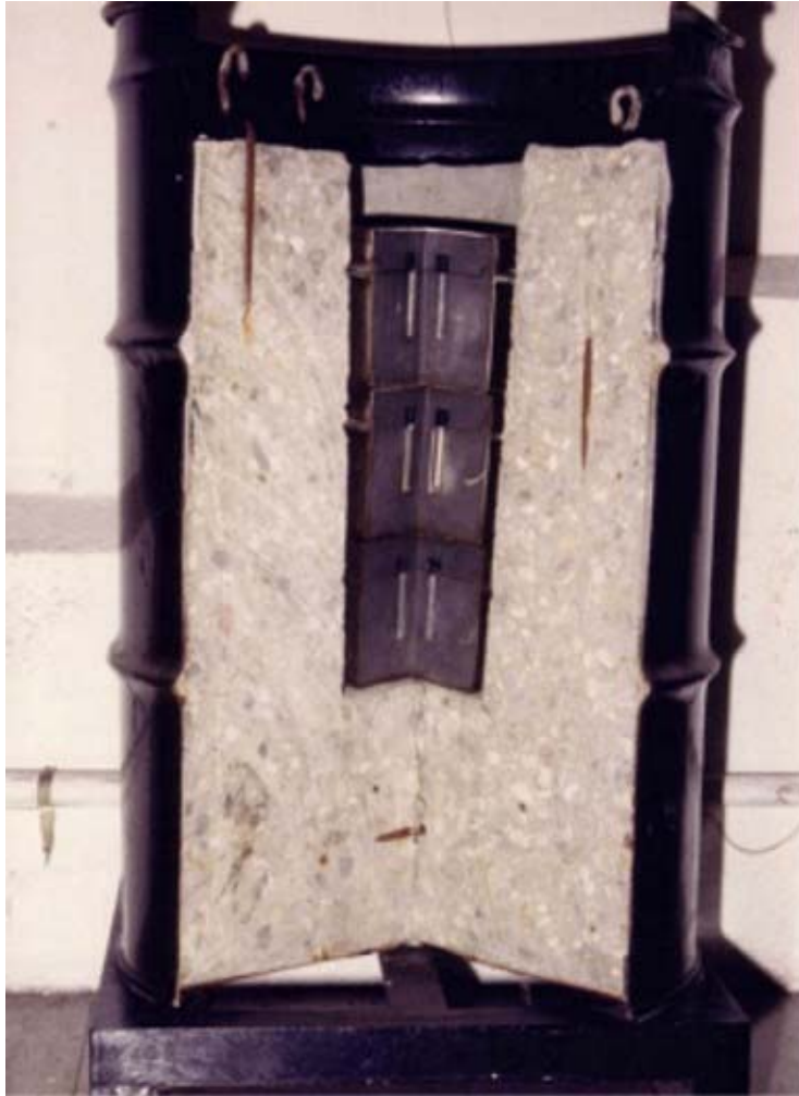
Figure 1. A mock-up of the Ra-226 sources finally conditioned and the aircraft used for their transportation to USA for final management
