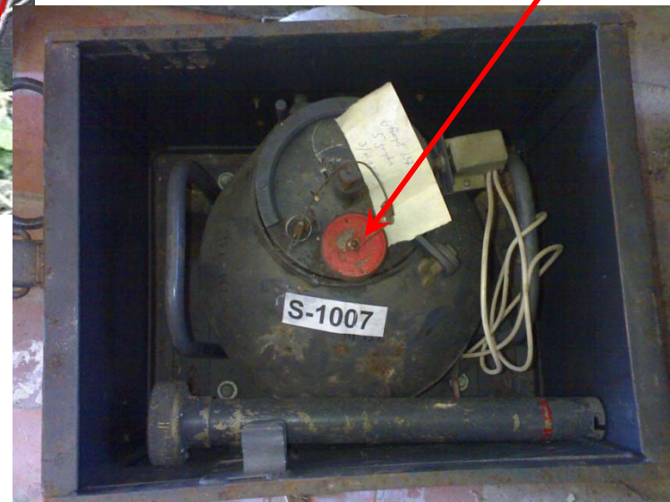
Typical container with ^{137}\text{Cs} source found on former military base
