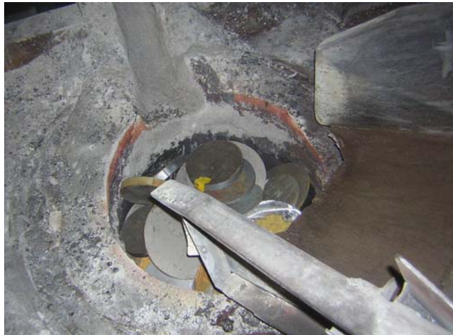
Pellets in the furnace Average activity : 10 bq/g
