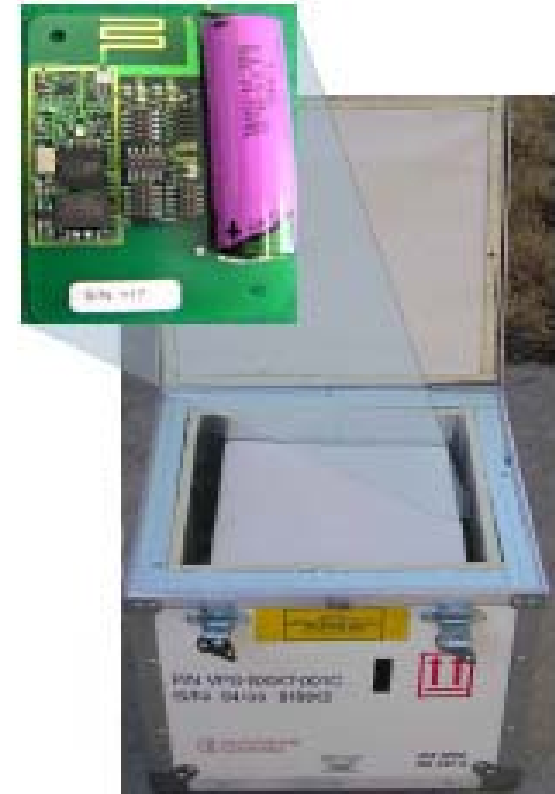
Modified Type A Radioactive Material Shipping Container: Wireless tag embedded in wall
