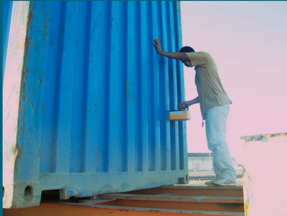
Dose measurement at the container surface
