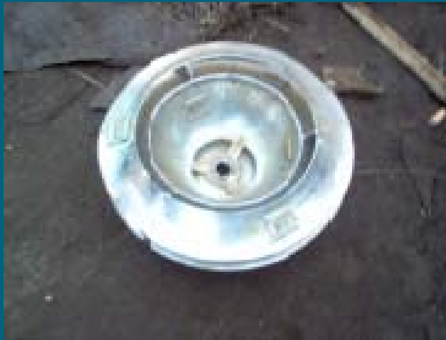
Figure 3: Isolated radioactive material (Lighting conductor with Ra-226 source)
