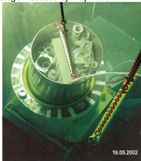
Conditioning of ILW - Under water loading of GNS-Mosaik Container
