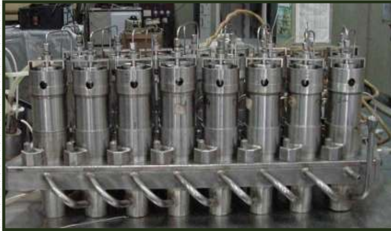
16 Stage Centrifugal Extractor Bank
