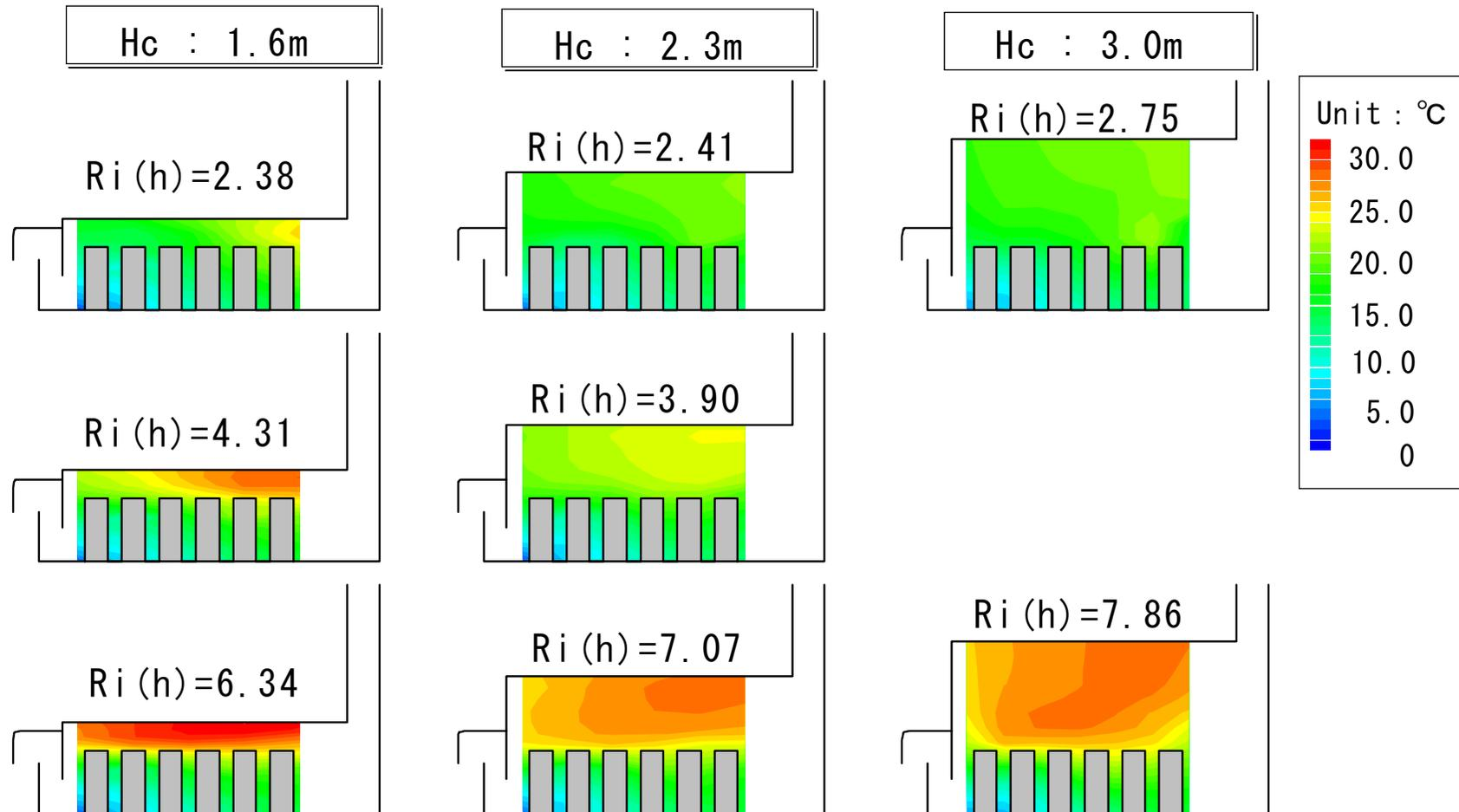
***The ceiling height and stack height directly influences the heat removal characteristic of the facility.***
