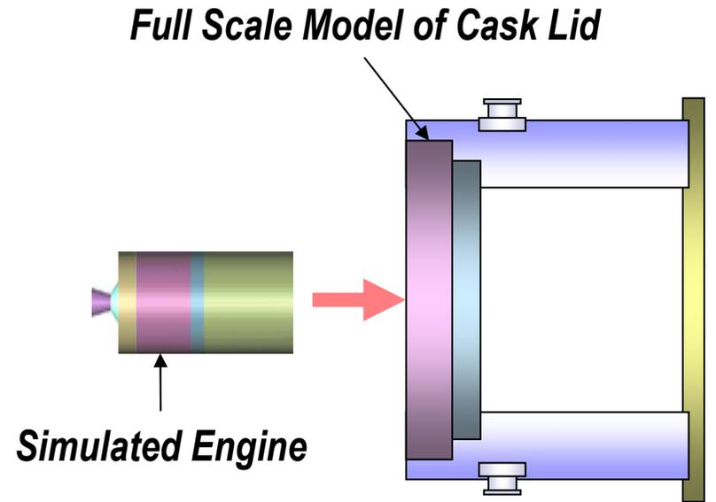
**Vertical crash test of full scale model cask lid crashed by a simulated engine (Nov. 2008)**
