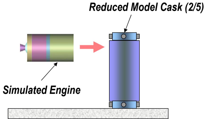
**Horizontal crash test of 2/5 reduced cask model crashed by a simulated engine (Jan. 2008)**
