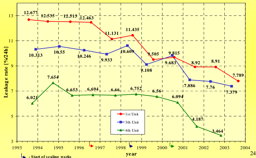
Leakage rate measured at Dukovany NPP
