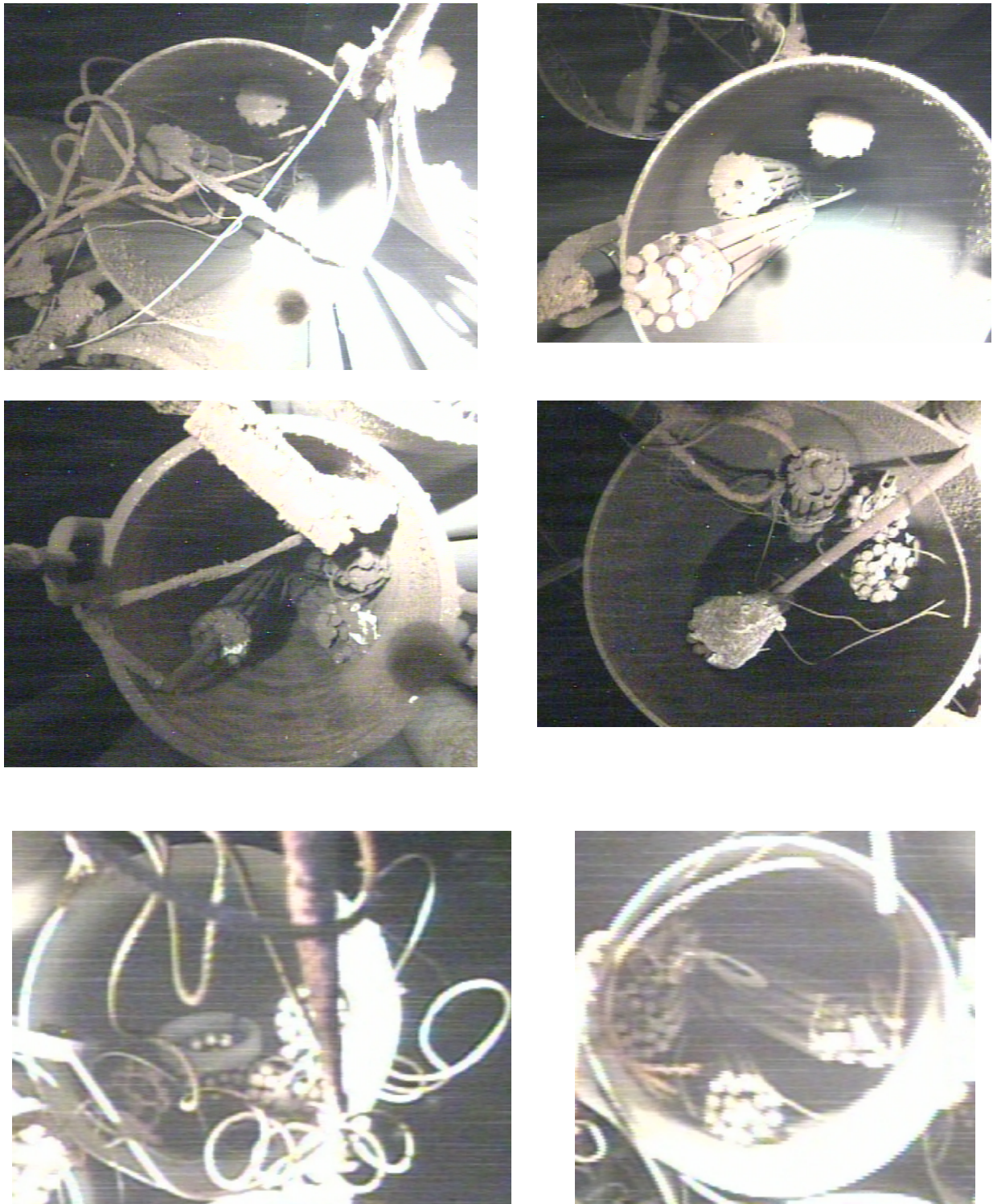
Figure 1 - Damaged Spent Nuclear Fuel in Special Canisters
