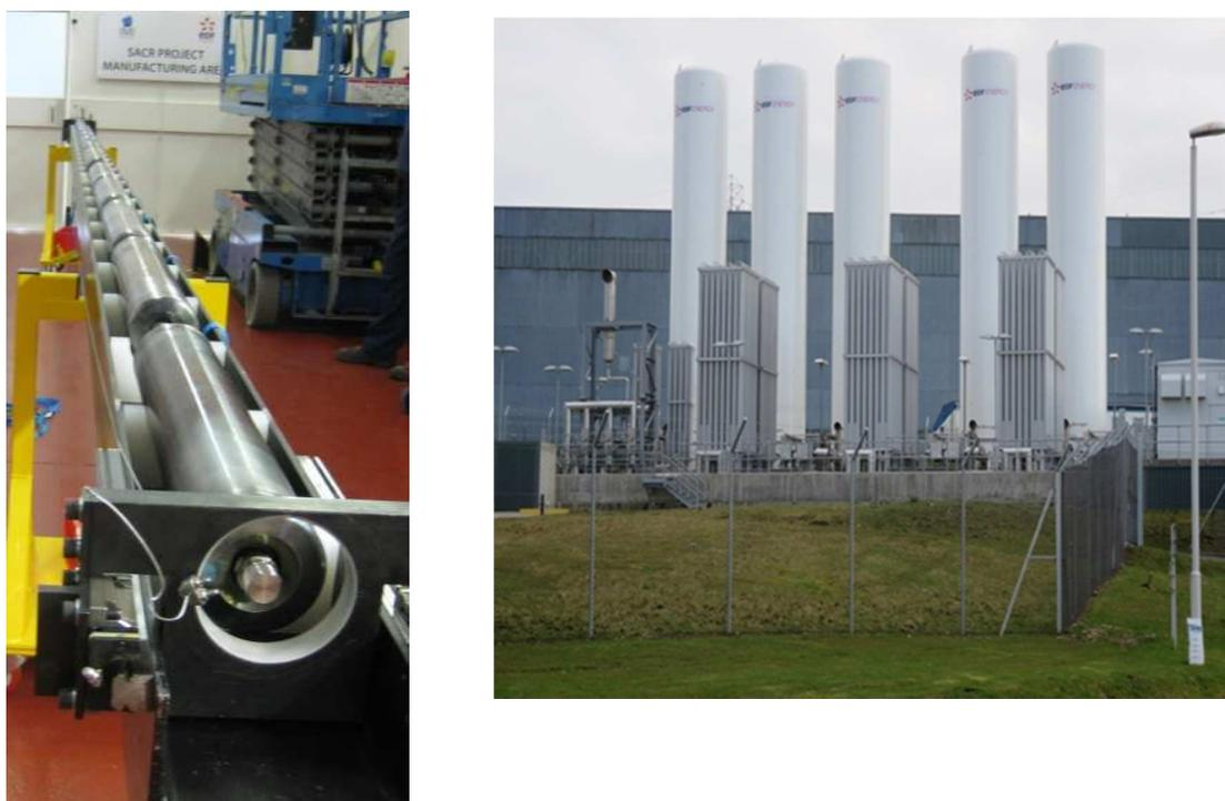
**Figure 5 – Super-articulated control rods and seismically qualified nitrogen system at Hinkley Point B reactors**
