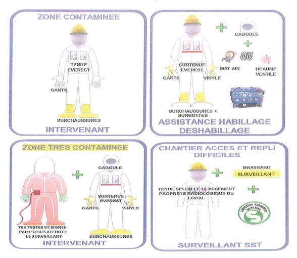
Clearly legible stickers provide a simple illustration of the equipment to be worn for entering the area (PPE + other appropriate equipment).
