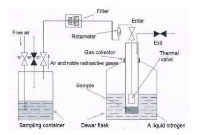
The measurement results of IRG specific activity in the primary circuit coolant present a reliable indicator for timely identification of microscopic fuel pin defects of "gas leak" type in the operating reactor core, and therefore are used as a valuable tool in fuel pin integrity monitoring during reactor plant operation at power.
