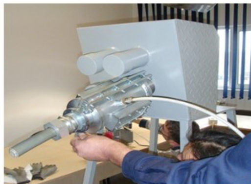
Figure 3 - Mock-up with vacuum box installed
