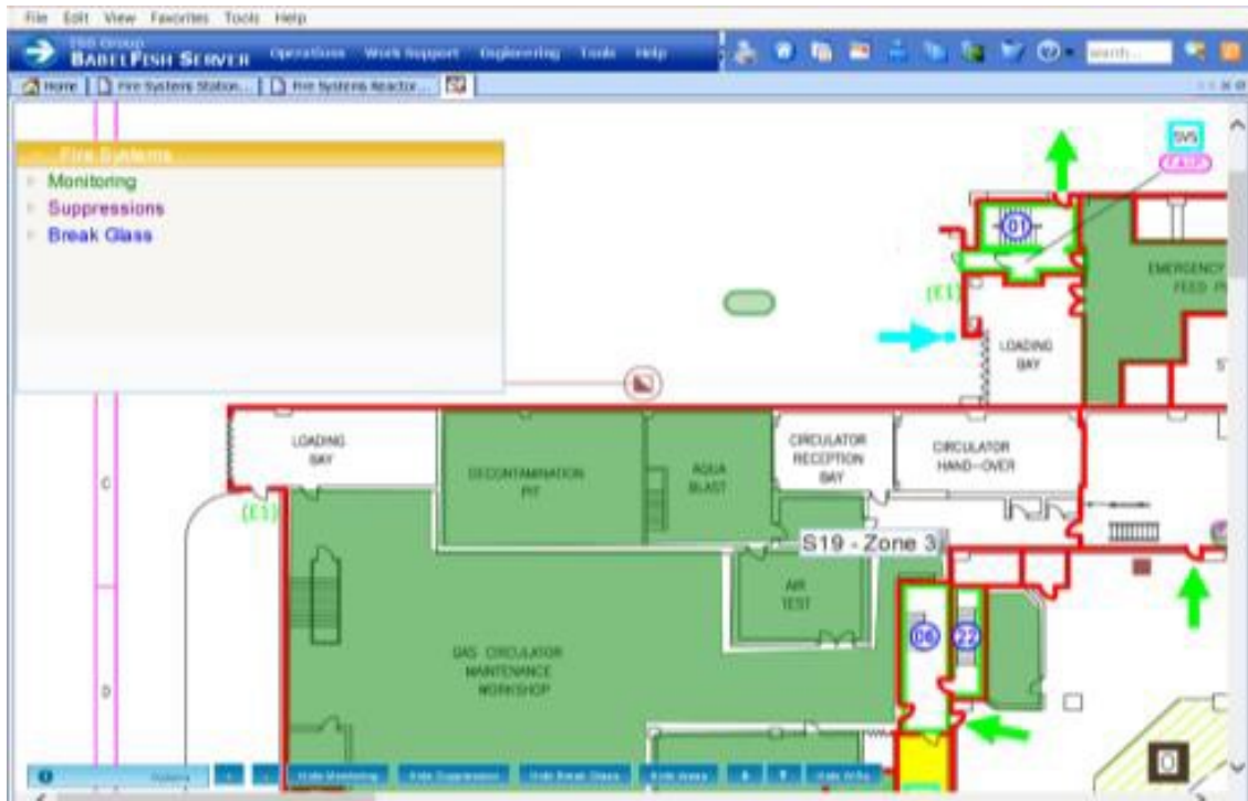
Figure 2: Detailed view of the Fire Station Systems Status in Maintenance Workshop Area
